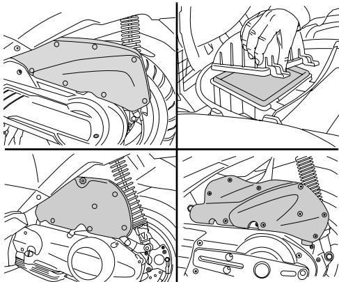
Replace the filter element <sup>2</sup>
