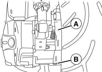
The gearbox must be drained when the engine is warm so that the oil will run easier.
