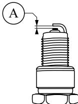
A. Electrode gap: 0.7 to 0.8 mm
